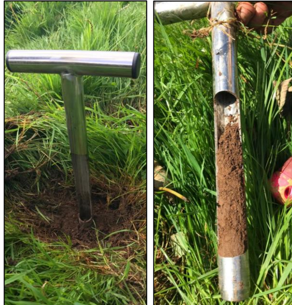
Figure 4: Picture of soil gouge used with vegetation scraped away in the P (left) and a sample to 15 cm depth (right), authors photography.
