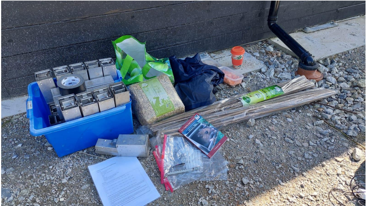
Figure 9. Small rodent survey equipment: 30 Longworth traps, label tape, straw bedding, bait (peanut butter & oat balls with carrot), bamboo canes, guidebook, plastic bags, methods sheet, fur clippers, Pelosa scale.
